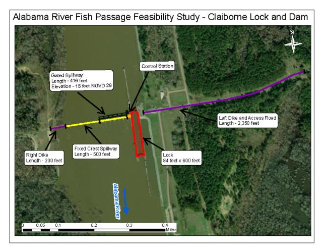
Figure 2: The Claiborne Lock and Dam
